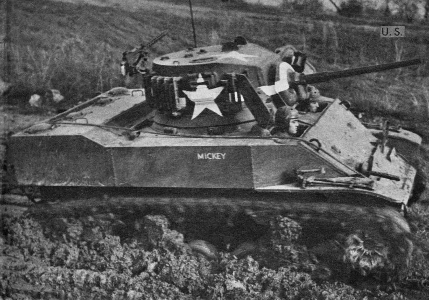
U. S. LIGHT TANK M-5, WITH ROUNDED TURRET, LED THE LANDING FORCE AT SICILY. HIGH, FLAT-TOPPED HULL IS RAISED AT BACK, ANGLED IN TOWARD FRONT
